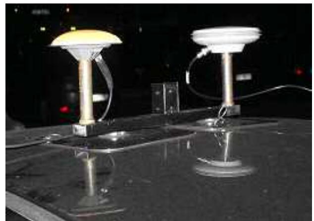
Figure 3 – Installation of the two rover receiver antennas on the car
