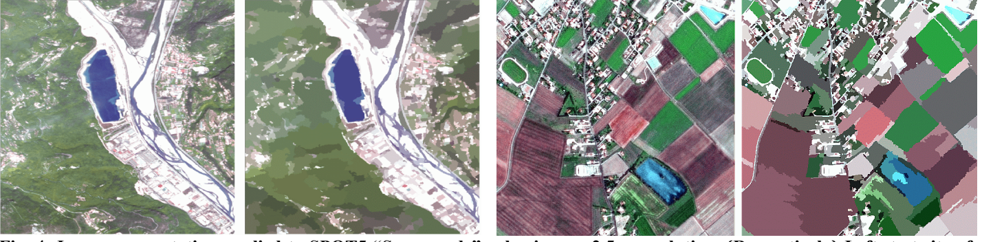
Fig. 4: Image segmentation applied to SPOT5 “Supermode” color image, 2.5m resolution. {Respectively} Left: test site of {Nice, Toulouse} (France), tile of {1024, 512}-pixel square. Right: segmented image obtained for {1500, 1300} regions.
