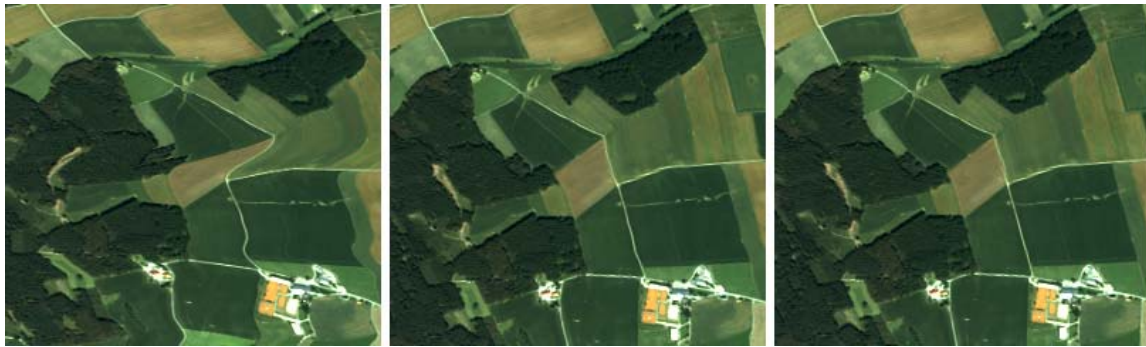
Figure 4: Effect of “moment of inertia” of the scan mirror on ortho image accuracy. The left image shows the original data, the middle image the uncorrected ortho image and the right image the corrected ortho image. The uncorrected ortho image (middle) shows undulated roads with respect to the corrected ortho image. This effect can be mainly observed for heavy roll movements and is different for the sensor systems (not all sensors show this effect).
