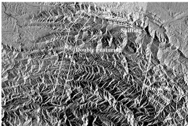
Fig. 1. Typical geometric problems in SAR
