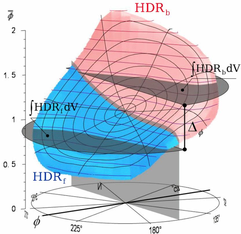
Figure 1. Two parts of the normalised to the nadir viewing hemispherical-directional reflectance *HDR* distribution of a soil surface, separated by the line perpendicular to a  $\phi$  direction, the  $HDR_b$  and the  $HDR_f$ , with their average values calculated as the  $\int HDR_b dV$  and the  $\int HDR_f dV$ , enabling us to compute the absolute value of the difference between them.
