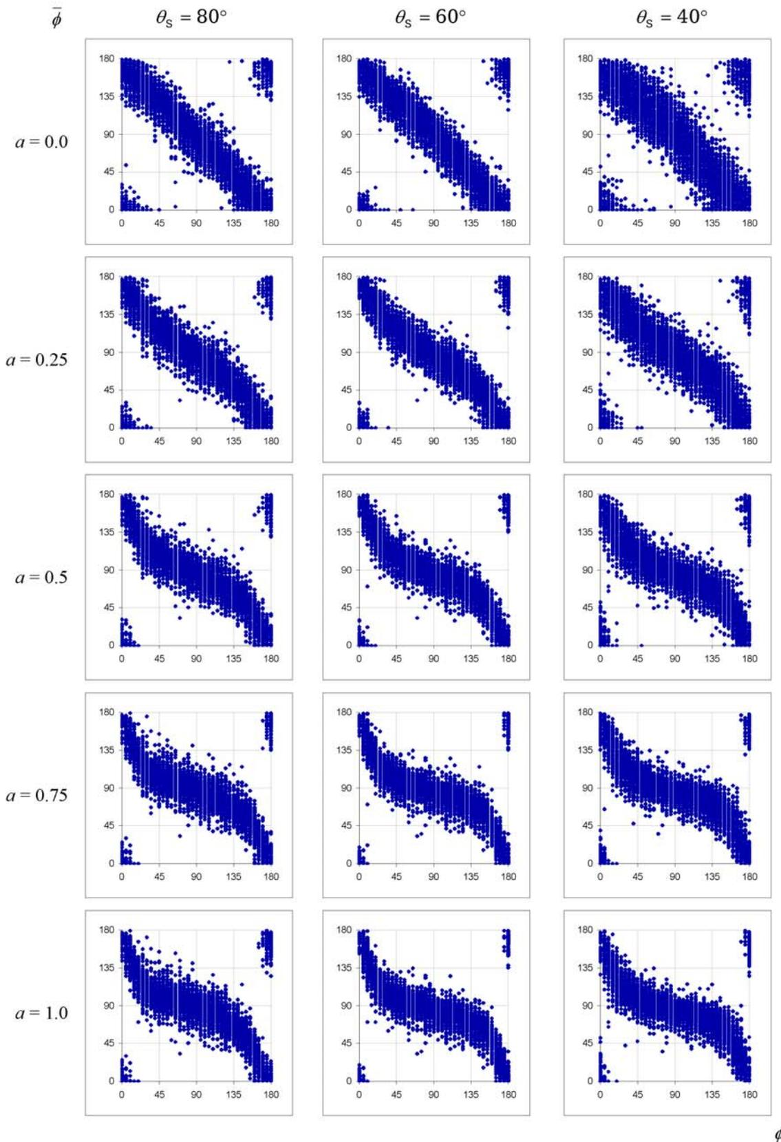
Figure 4. Relation between the angle  $\bar{\phi}$  for which the  $\Delta_{\phi}$  reaches its maximal value and the angle  $\phi_{s,c}$  describing the illumination of their furrows as a distance angle between the direction of the furrows and the sun position, established for five soil surfaces with various clarity of their furrows described by the parameter  $\alpha$ , illuminated at specified solar zenith angle  $\theta_s$ .
