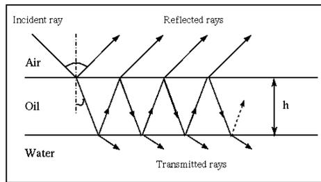
Figure 3: Multiple reflections across an oil film as described by a thin layer optical model
