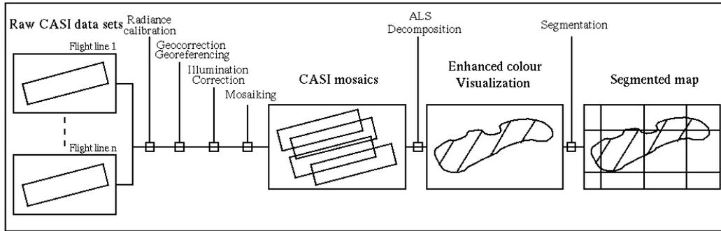
Figure 1: CASI data processing chain
