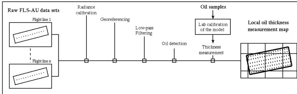
Figure 5: FLS-AU data processing chain
