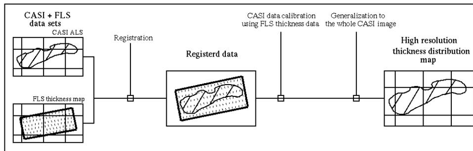
Figure 7: CASI + FLS-AU data fusion chain
