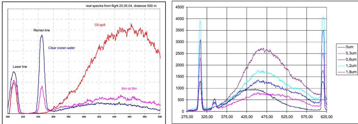
Figure 6: (left) FLS-AU spectra recorded during the DEPOL04 experiment over water and oil films (right) Spectra used in the lab for calibrating the thickness estimation model
