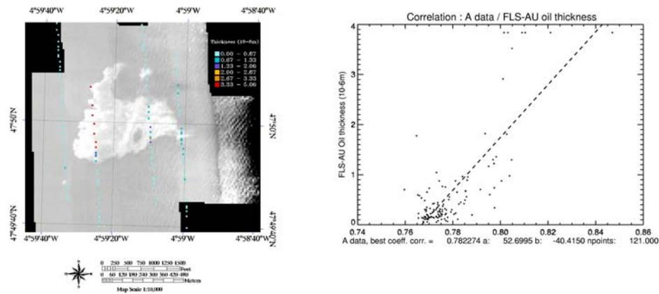
Figure 8: (left) Registration of CASI data with thickness measurements from FLS-AU; (right) Absolute calibration of CASI data using corresponding FLS-AU estimated thicknesses
