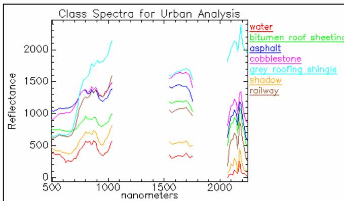
Figure 3: Urban analysis: Class spectra of selected man-made materials, water and shadow
