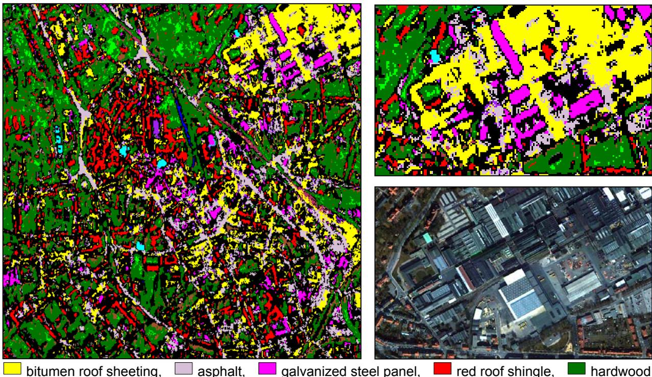
Figure 8: Combined classification results from MNF- and DBFE-transformed datasets. The subset of the upper right edge shows an industrial area with mostly bitumen-roof-sheeting-covered buildings and some asphalted streets and parking areas around.
