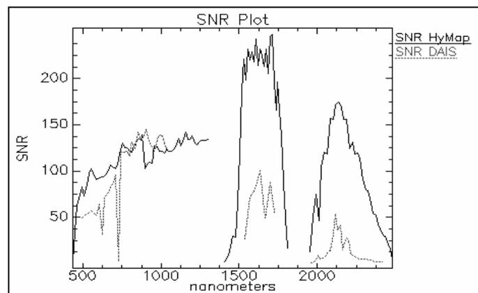
Figure 2: Comparison of the Signal-to-Noise-Ratios (SNR) of DAIS 7915 and HyMap
