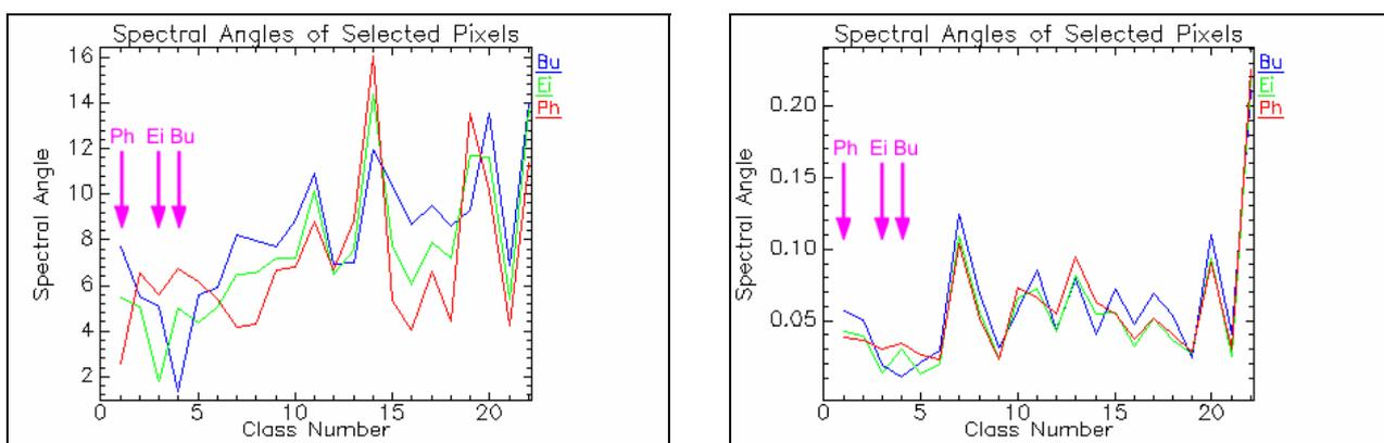
Figure 10a + b: Plot of calculated spectral angles for three selected pixels in the original (a) and DAFE-transformed (b) feature space. Arrows indicate the class numbers of the three tree species where the lowest spectral angle should appear for correct classification.
