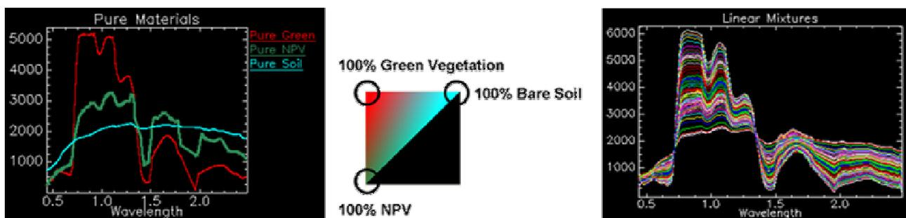
Figure 5: Illustration of synthetic scenes. Left: Input spectra of pure materials. Center: Synthetic image based on linear mixture of the input spectra. Right: Example for simulated mixed spectra.
