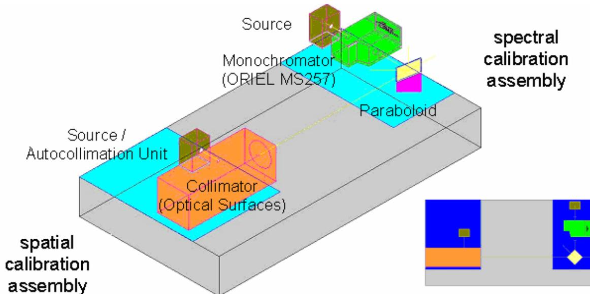
Figure 3: Oblique view and top view (right insert) of the working spaces on the calibration bench
