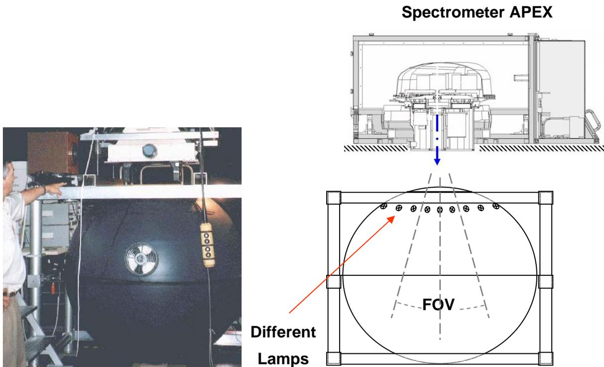
Figure 4: Picture and principle of the radiometric calibration of APEX imaging spectrometer using a large integrating sphere
