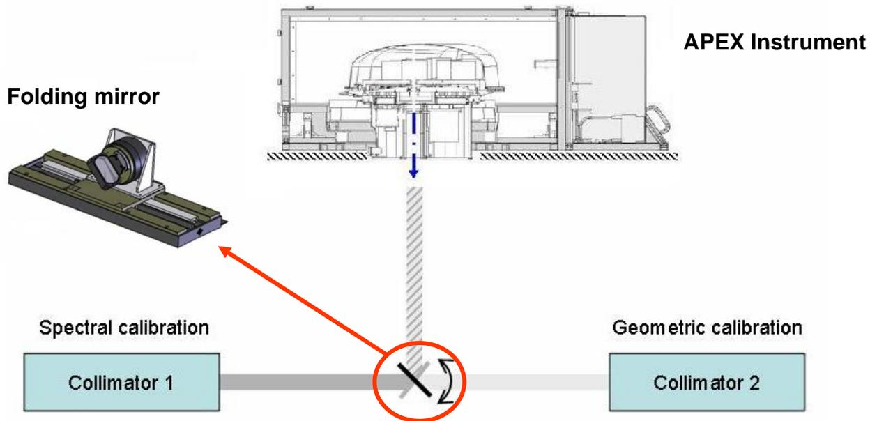
Figure 2: Schematic view of a set-up with fixed APEX instrument, fixed collimators and movable/flapping folding mirror.
