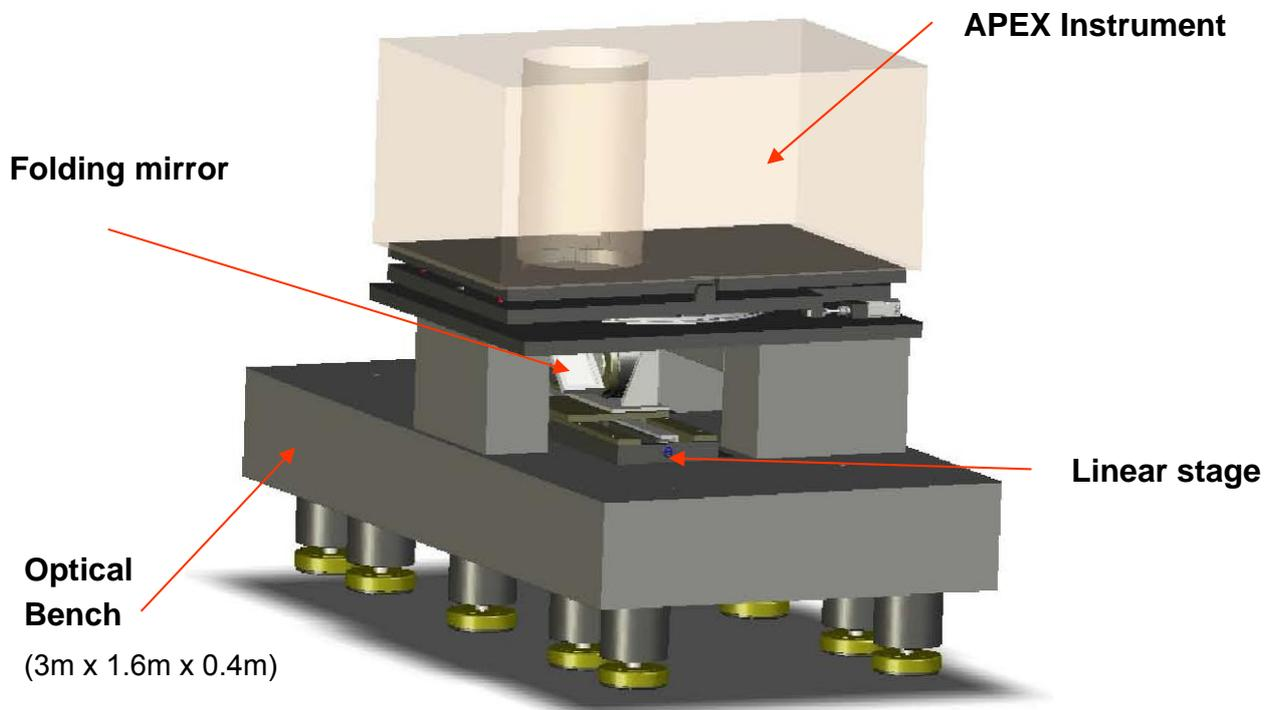
*Figure 1: Side view of the calibration bench with the APEX sensor, the two working areas on both sides and the folding mirror*
