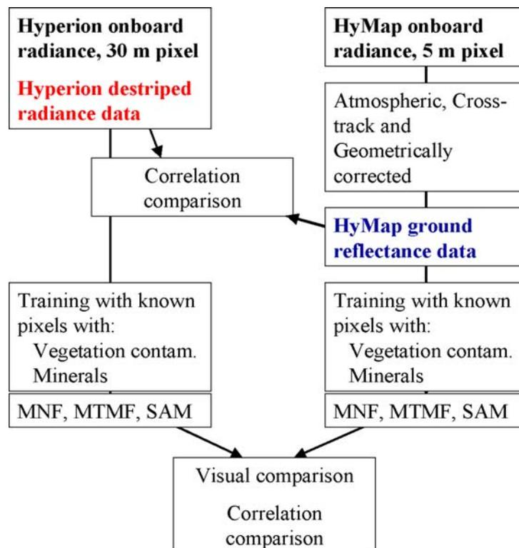
Figure 4 Flow chart of image processing and comparison. The acronyms are explained in the text.
