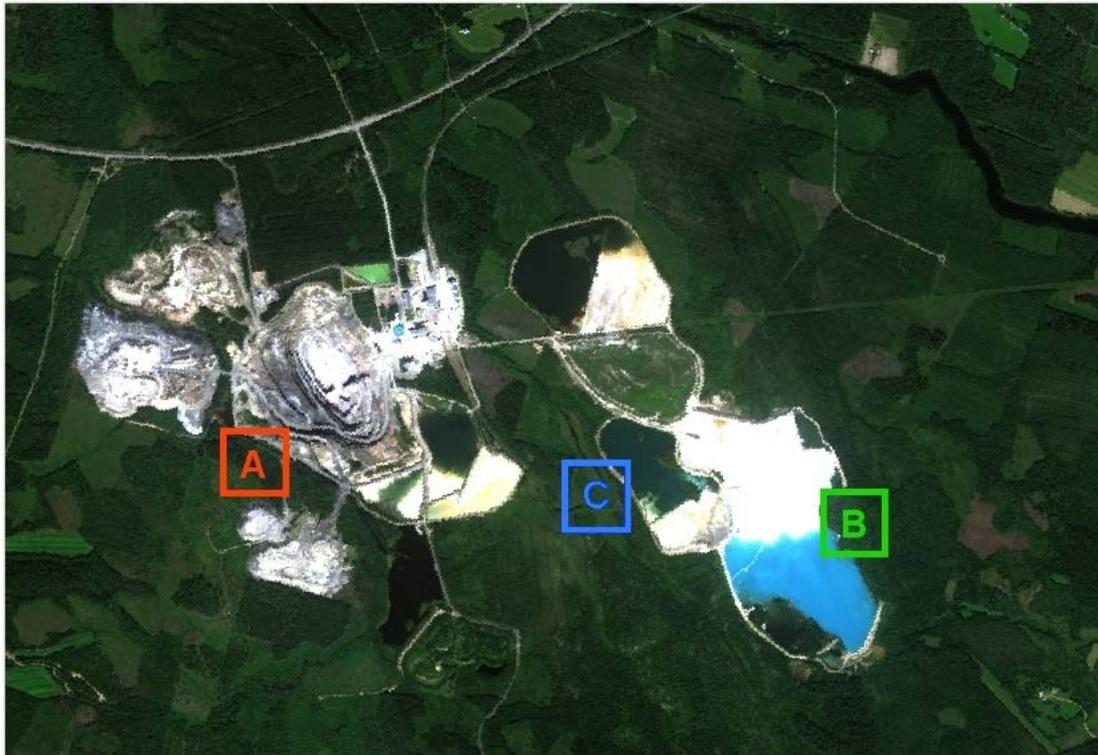
*Figure 2 Color composite picture of visual (red, green and blue) channels of the HyMap airborne image data from the Lahnaslampi area. The open pit, enrichment plant, waste rock piles and the tailing ponds are visible. Pixel size is  $5 \times 5 \text{ m}^2$ . The training sites are marked by the coloured squares A, B and C. Width of the area is 4 km. Recorded on 28<sup>th</sup> July 2000.*
