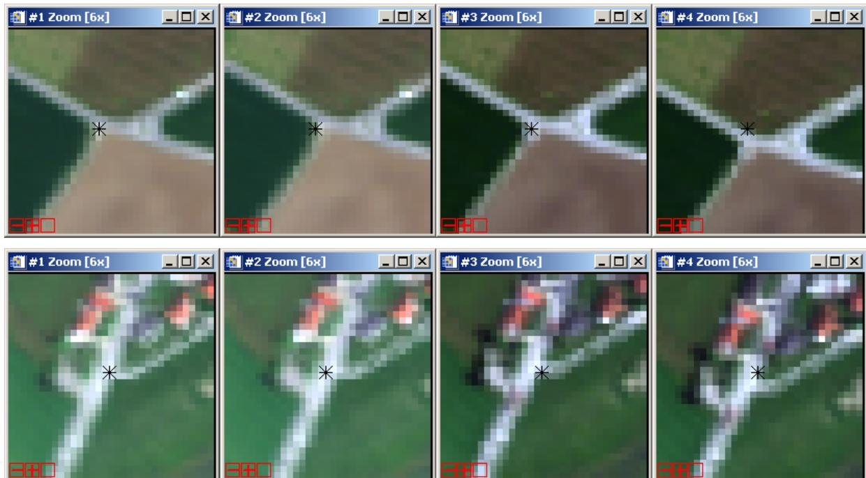
Figure 7: Result of ortho-rectification. 1<sup>st</sup> and 2<sup>nd</sup> column: HyMap scene 1 26.05.2004, left with GCPs, right with mean boresight misalignment angles. 3<sup>rd</sup> and 4<sup>th</sup> column: HyMap scene 2 26.05.2004, left with GCPs, right with mean boresight misalignment angles
