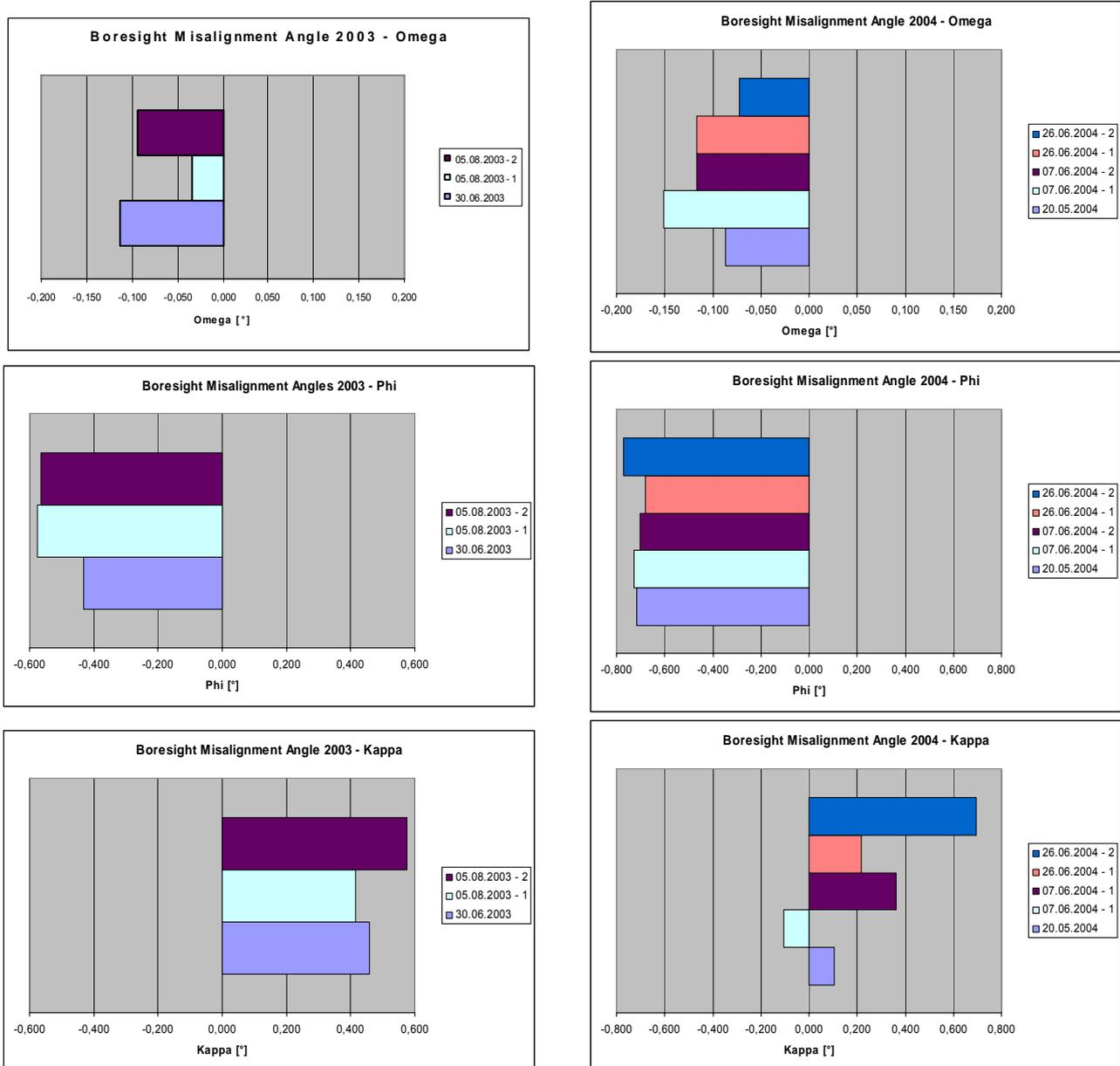
Figure 4: Boresight misalignment angles determined in 2003 and 2004 (units: degrees)
