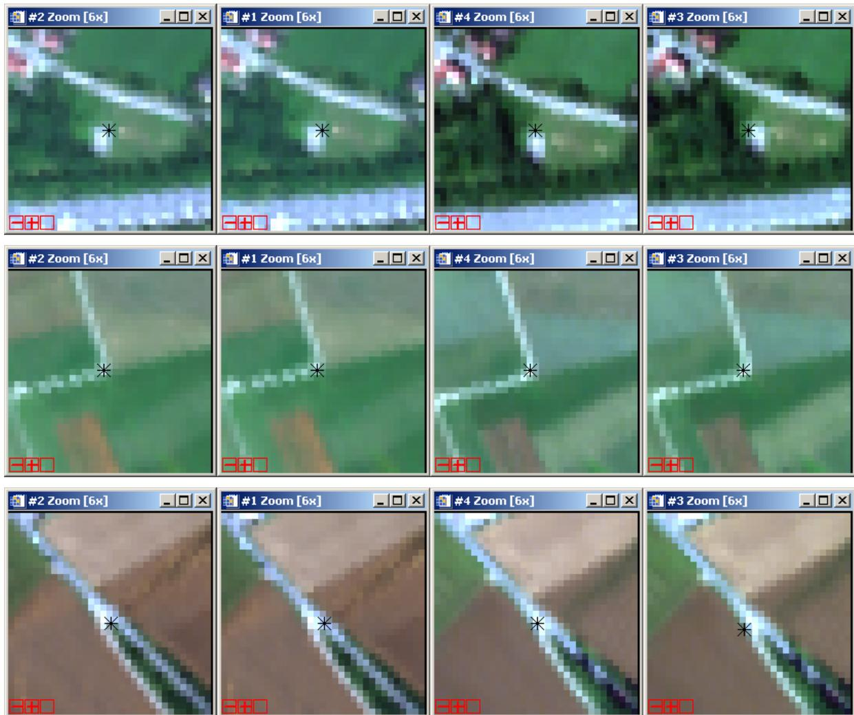
Figure 6: Result of ortho-rectification. 1<sup>st</sup> and 2<sup>nd</sup> column: HyMap scene 22.07.2003, left with GCPs, right with mean boresight misalignment angles. 3<sup>rd</sup> and 4<sup>th</sup> column: HyMap scene 15.07.2003, left with GCPs, right with mean boresight misalignment angles
