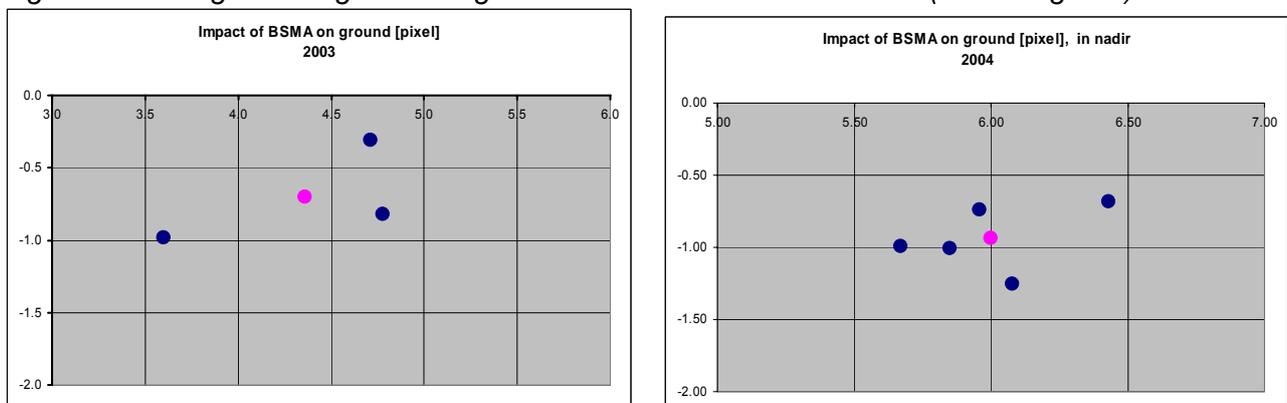
Figure 5: Impact of boresight misalignment angles on nadir position (values of 2003 and 2004, units: pixel)
