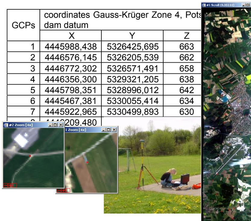
Figure 1: Calibration field close to Oberpfaffenhofen with its Ground Control Points surveyed with differential GPS
