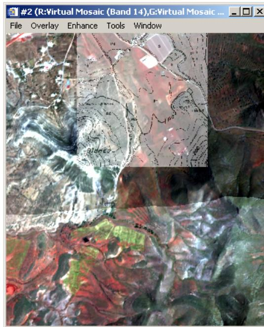
Figure 9: Mosaic of two ortho-rectified HyMap scenes of Cabo de Gata (Spain), where the mean BSA was used as input for ORTHO. The mosaic is partly overlaid by a topographic map.
