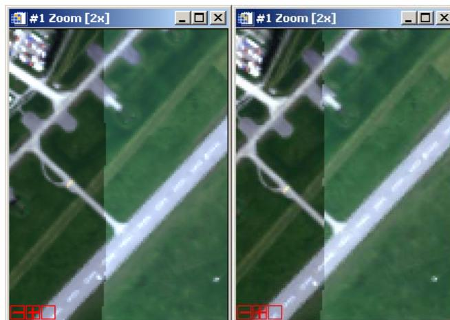
Figure 8: Mosaic of scene 1 and 2: left with GCPs, right with mean boresight misalignment angles
