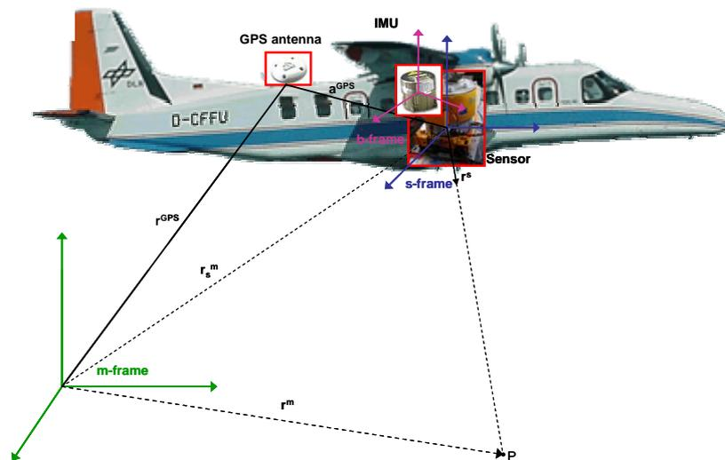
Figure 2: Detailed diagram of elements of direct georeferencing for the airborne case (e.g. HyMap)
