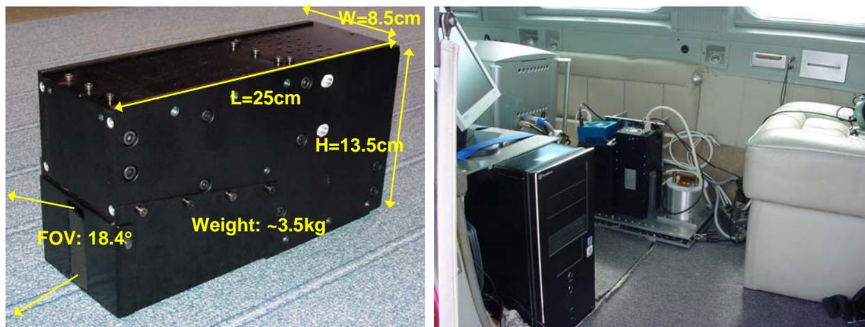
Figure 1 The VNIR-640 instrument (left) and the VNIR-1600 and SWIR 320i mounted in a plane with IMU (right)
