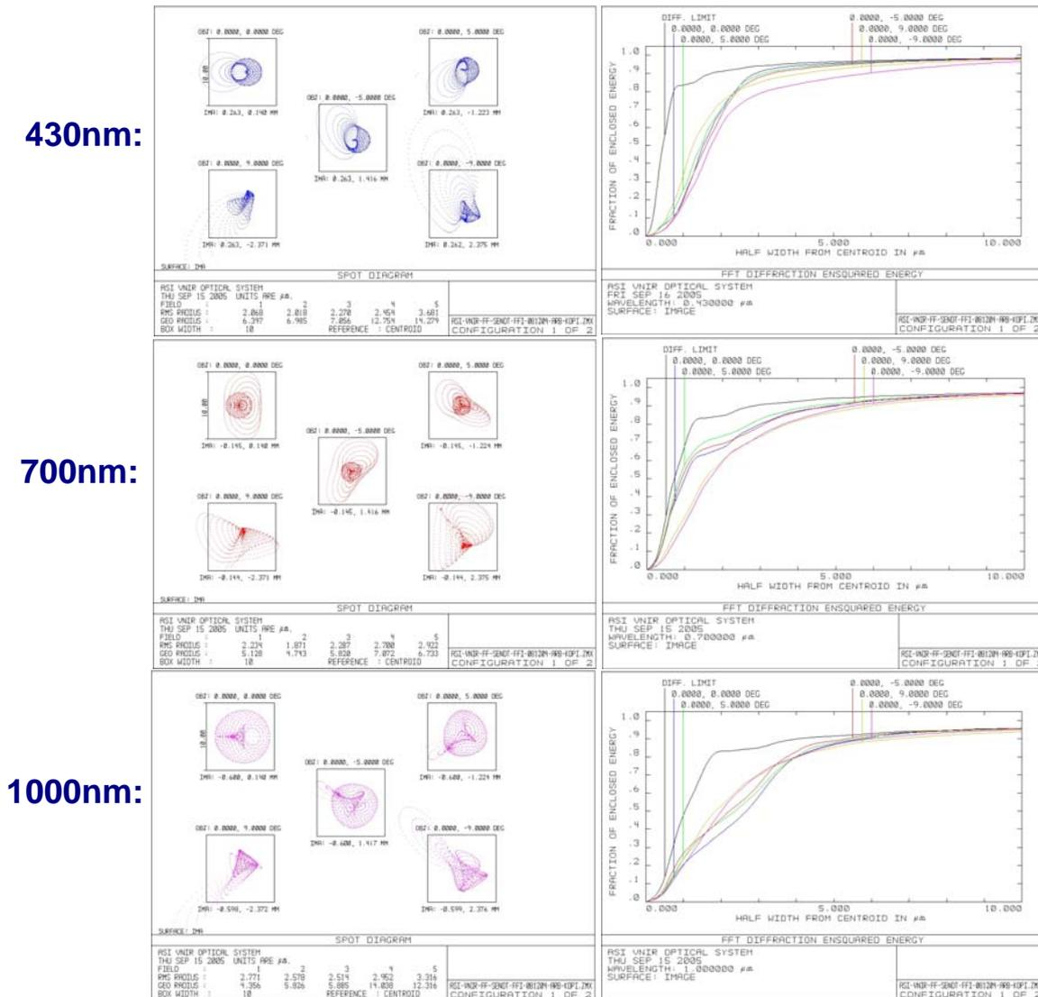
Figure 2 Spot diagram (left) and ensquared energy diagrams (right) for different wavelength and fields of view for the VNIR-640 module.
