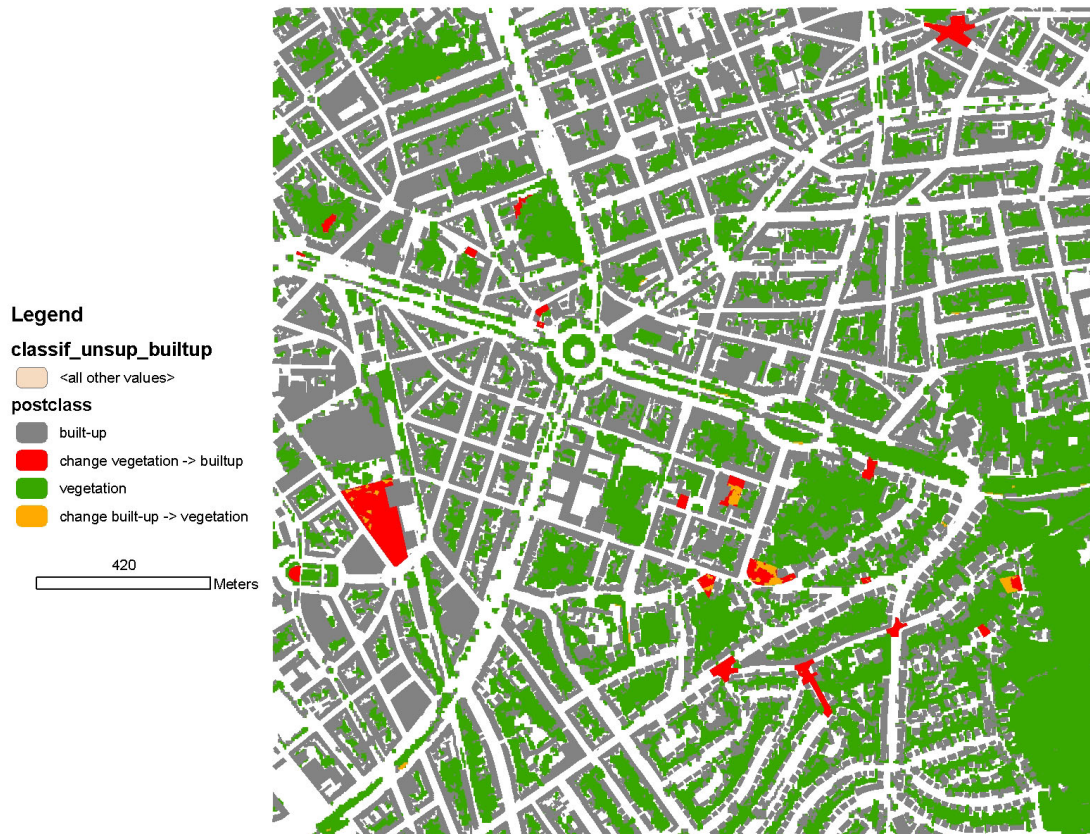
Figure 9: overlay of the masks with the unsupervised classification of the multi-temporal composition. In green: unchanged vegetation area, in grey: unchanged building areas, in red: changed areas from vegetation to building areas, in orange: changed areas from buildings to vegetation.
