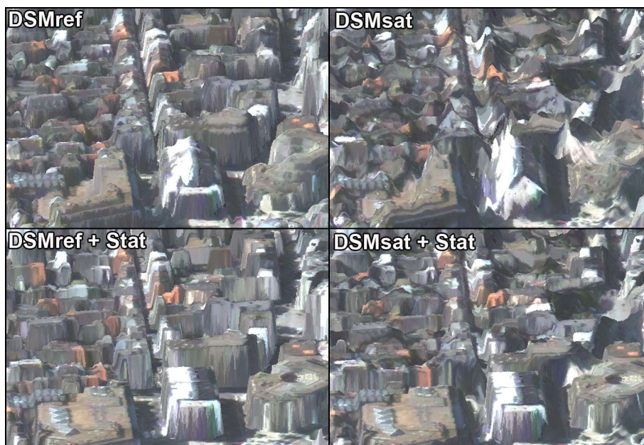
Figure 6: 3D views based on various DSM (LIDAR on the left and Satellite on the right) and on the extrusion process (below)
