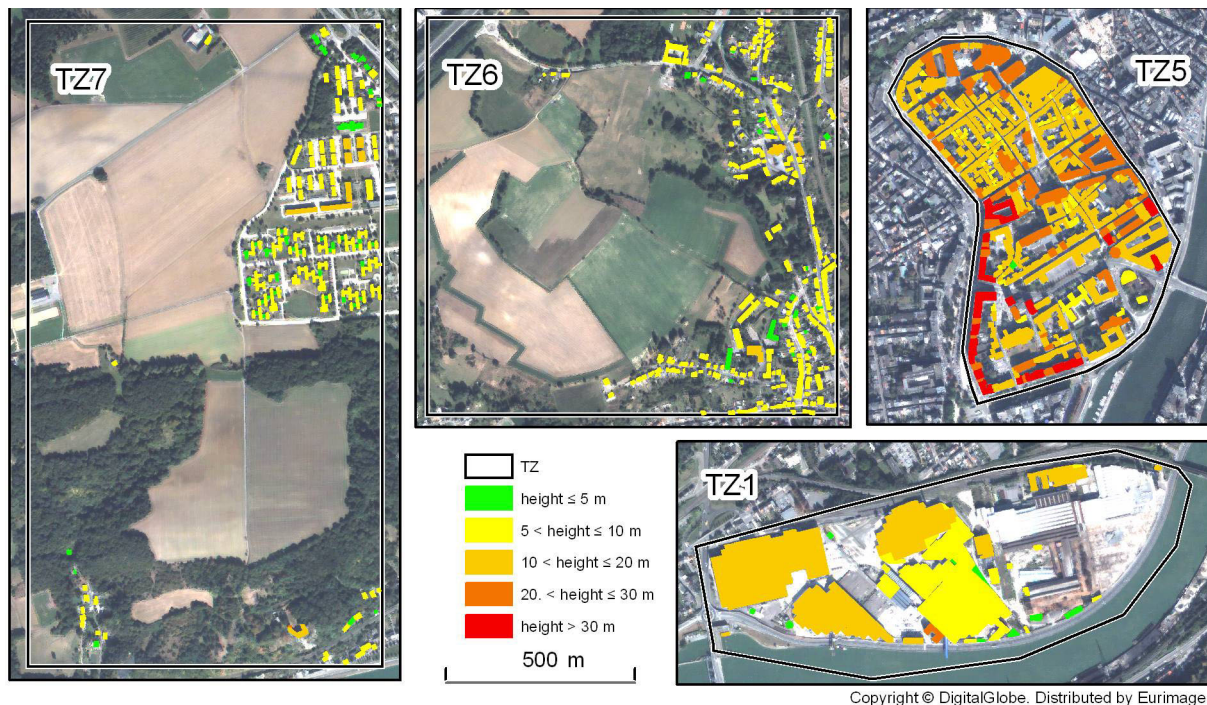
Figure 2: Classification of the building heights computed in the different test-zones from reference data
