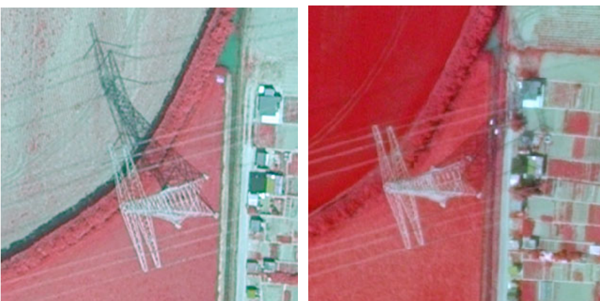
Figure 5: Shadows in different directions due to sun angle differences
