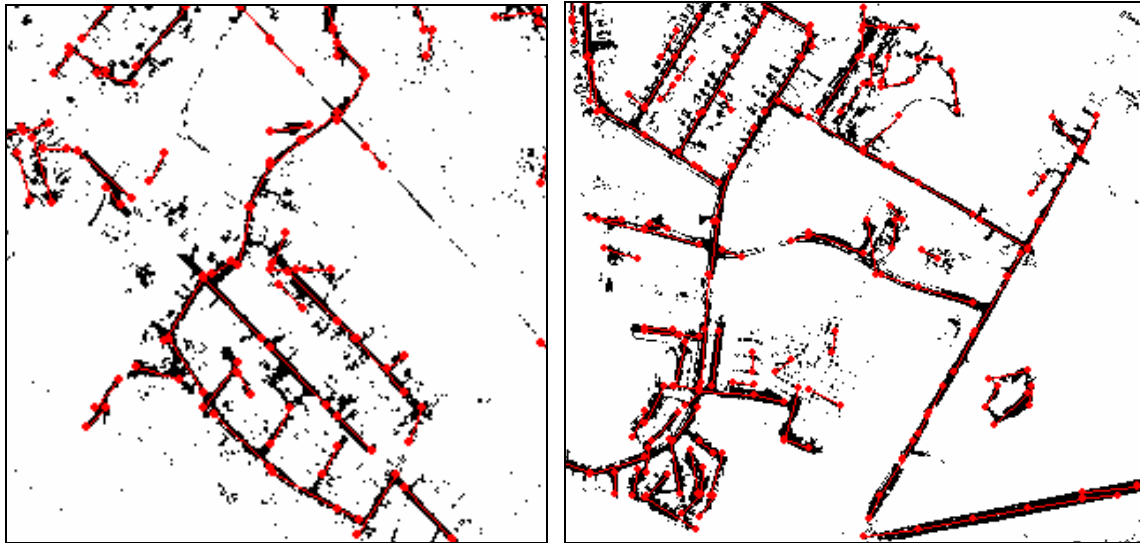
Figure 5: Road centreline extraction: extracted road centreline segments (red) overlaid on classified road pixels (black) from the Ikonos test image (left) and the Quickbird test image (right)
