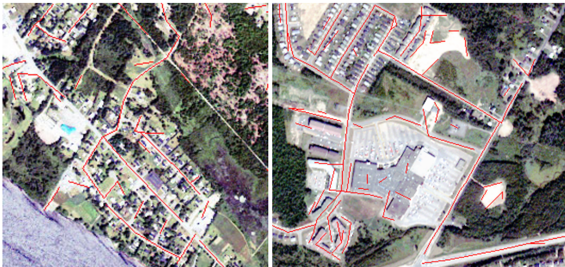
Figure 6: Road network formation: final road networks (red) overlaid on the original Ikonos test image (left) and the original Quickbird test image (right)
