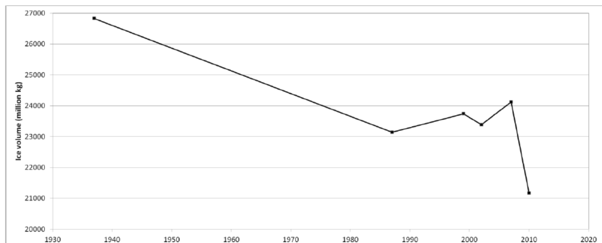
Figure 8: Change in volume of Sørfonna measured by comparing DEMs generated from digitised contour lines, ASTER images and provided pre-prepared. The volume trend shows the same trend as glacier area albeit not at
