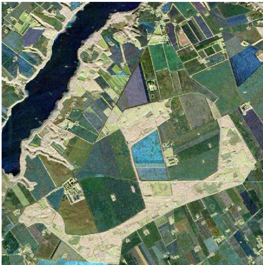
Figure 2: L-band RGB image ( R is HV , G is HH and B is VV ), 16 August 1998; 5,120 m by 5,120 m.
