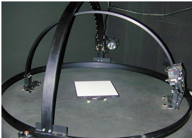
Figure 1: Mechanical system setup of CLabSpeG: Horizontal aluminum rail supporting the light source arm, which rotates anti-clock wise with a resolution of 30 degrees; Stationary arm supporting the imaging sensor with a resolution of 15 degrees in zenith; Sample holder in the centre with a spectralon panel on top, rotating clock-wise with a resolution of 30 degrees.
