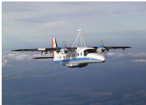
Figure 4: Dornier 228-101, D-CODE in configuration for project HYLTEC (camera on stand, camera at the wing, device to measure number of insects under the wing)
